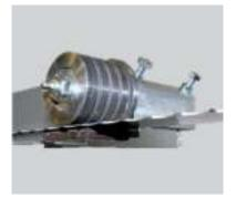
When cutting the saw band is guided by hardened and ground guide pulleys. When before the cut, it is additionally guided in combination with precise hard-metal guidance. This system can be fully adjusted in all directions and it ensures optimum position of guide pulleys and the saw band.
