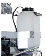
Gravity cooling and lubricating of the band with adjustable outlets in both guide pulleys ensure that the saw band is in optimum condition during cutting.
