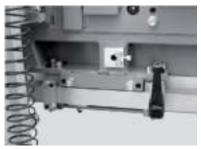
In order to ensure accuracy of the cut the guide pulley on the operator's side moves as close as possible to the workpiece. Simply operated massive bearing system. It can be motor-powered and controlled as an auxiliary device from the control panel.
