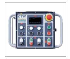
The feed into the cut and back is driven by an electric motor with worm gearbox controlled by a frequency converter. You can change the speed of travel simply by turning the potentiometer on the control panel. End positions are secured against impact by means of limit switches with automatic deceleration and stopping.
