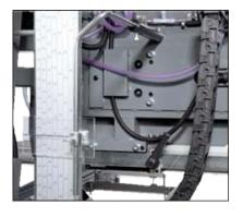
In order to ensure accuracy of the cut the guide pulley on the operator's side moves as close as possible to the workpiece. Simply operated massive bearing system. It can be motor-powered and controlled as an auxiliary device from the control panel.
