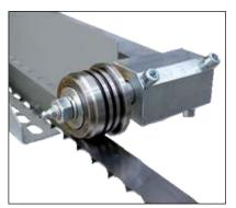
The saw band is guided in the cut by hardened and ground guide pulleys. This system can be fully adjusted in all directions and it ensures optimum position of guide pulleys and the saw band.
