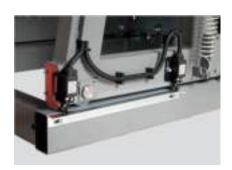
Both ends of the guides are fixed on both ends against the bridge collision with 2 limit switches. It will slow down and then stop the bridge.
