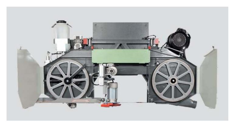
The arm is fitted with blade wheels made of high-quality grey cast iron with accurate balancing against vibrations. The wheel has a groove along its circumference. The groove holds a replaceable rubber-textile belt which creates an opti- mum contact area between the wheel and the saw blade.
