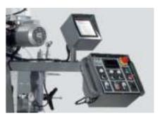
The design of the arm (now 40 kg heavier) and the sliding hard chromium rods has been reinforced. Due to heavier weight, the motor is now equipped with a brake, as in machines of the highest category. It significantly increases the accuracy of stopping at the desired point and contributes to the service life of the whole uplift system.
