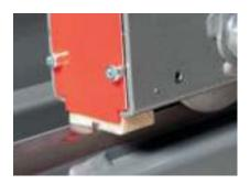
Felt wipers causes precise cleaning of rail strips
